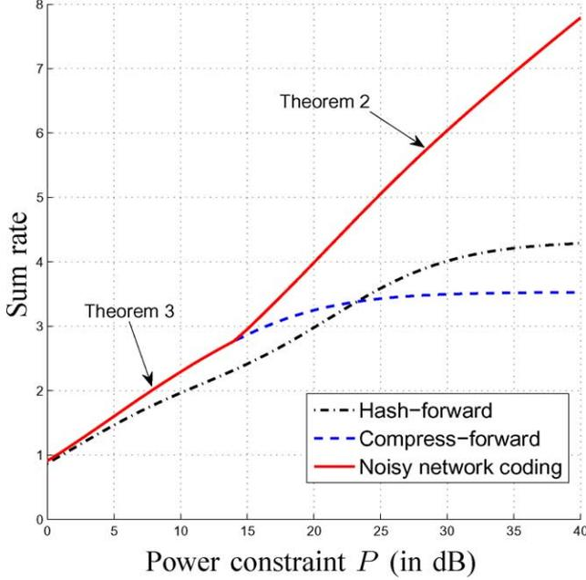
Fig. 4. Comparison of coding schemes for  $g_{41} = g_{52} = 1$ ,  $g_{51} = g_{42} = g_{31} = 0.5$ ,  $g_{32} = 0.1$ ,  $R_0 = 1$ .
