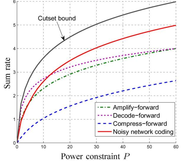
Fig. 2. Comparison of coding schemes for  $g_{21} = g_{12} = 0.1$ ,  $g_{31} = g_{23} = 0.5$ , and  $g_{32} = g_{13} = 2$ .
