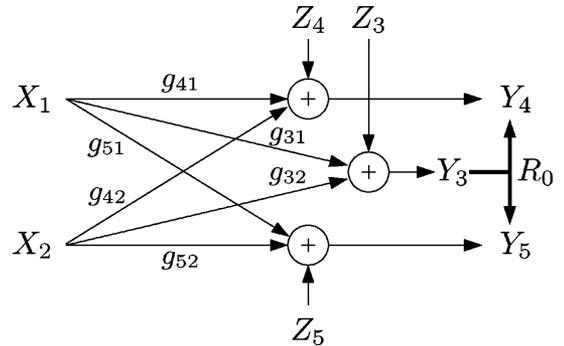
Fig. 3. Gaussian interference relay channel.
