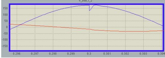
Fig. 3. The data shows how the local impedance controller manages substantial reactive loads, without Q compensator in the system.
