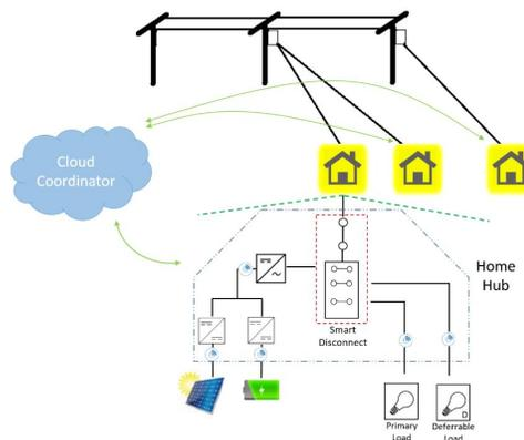
Fig. 1. Powernet's deployment within the legacy grid.
