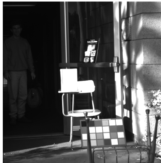
Image using DR=48dB sensor at t_{int}/4
