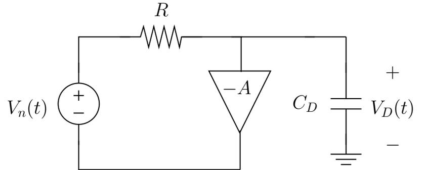
$\frac{V_D(f)}{V_n(f)} \approx \frac{1/A}{1+j2\pi f\left(\frac{RC_D}{A}\right)}$ $\overline{V_D^2(t)} = \frac{kT}{AC_D}$ |
