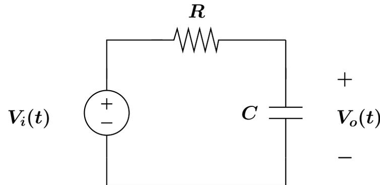
$V_i(t)$  is the thermal noise associated with  $R$  and is a WGN process with  $S_{V_i}(f) = 2kTR$ . Find the average output power  $\overline{V_o^2(t)}$
