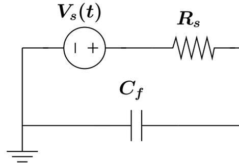
In this case, no noise is stored on  $C_b$  and the noise stored on  $C_f$  has average power  $\frac{kT}{C_f} = 20.7 \times 10^{-8} \text{V}^2$  and is transferred to the output during readout
