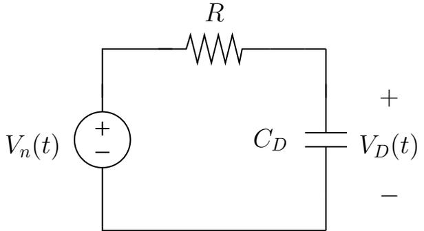
$\frac{V_D(f)}{V_n(f)} = \frac{1}{1+j2\pi fRC_D}$ $\overline{V_D^2(t)} = \frac{kT}{C_D}$ |
