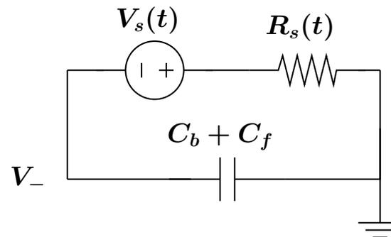
In this case noise is stored on both  $C_b$  and  $C_f$ , and its average power is  $\frac{kT}{(C_b + C_f)}$
